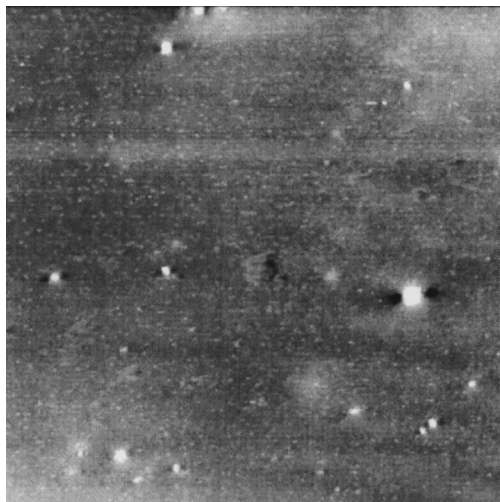
Fig. 1. Topographic image of unfilled uniaxial film. Image size 20\ \mu\text{m} \times 20\ \mu\text{m} . Contact mode with MUA-functionalised probe tip. Z-scale range 0–20 nm.
